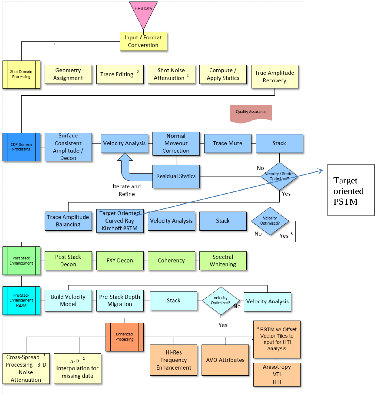
Generalised Land Seismic Processing Flow
